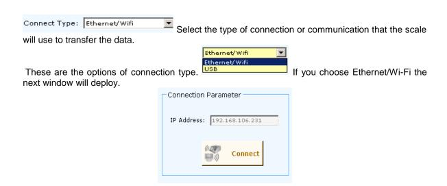
IP Address: 192.168.106.231 For Wireless or Ethernet, here you must specify the IP address you will assign to the scale for communicate with it.
